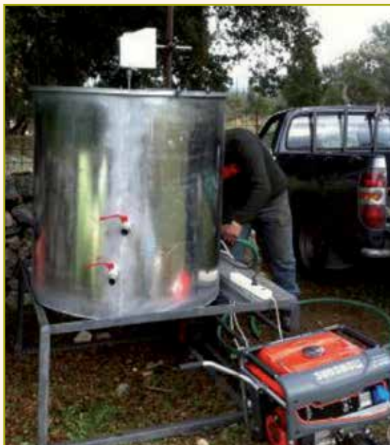
Photo 18. Tank with operating capacity of 0.5 m 3 with two valves on the side and one at the bottom, pump and generator.
