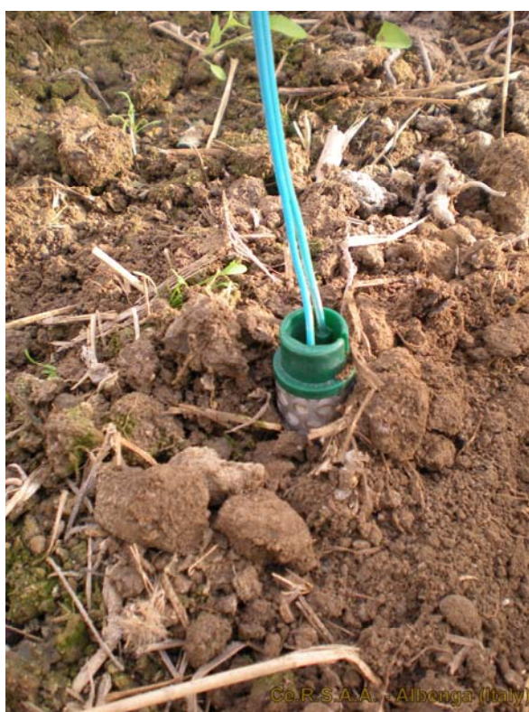
Figure 37: Tensiometer for the measurements of the soil moisture (Albenga, Liguria, Italy). (Source: Ce.R.S.A.A., 2010)
